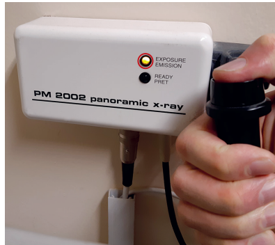
Figure 2.2 Examples of X-ray equipment warning devices with a suitable 'X-rays' indication (circled in red)
